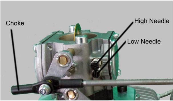
After fitting the engine into the model and after installation of the ignition, you can start the engine. (Note: Installation of the ignition must be in accordance with the manufacturer's directions.)
